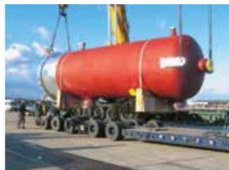
Turbine Cooling Air Cooler for GTCC plant
